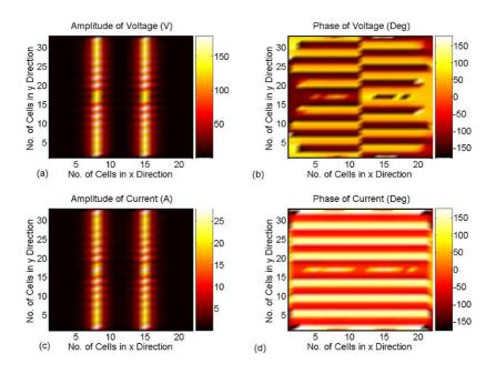
The voltage and current distributions on the TL-metamaterial superlens for two sources computed by TMM, where 21 × 33 unit cells have been used. (a) The amplitude distribution of voltage. (b) The phase distribution of voltage. (c) The amplitude distribution of current. (d) The phase distribution of current.
