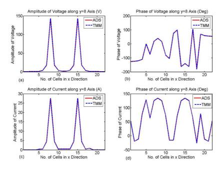
The amplitudes and phases of voltages and currents along the line y = 17 in the superlens for two sources, where the red lines are ADS simulation results and the dashed blue lines are TMM computation results. (a) The amplitudes of voltages. (b) The phases of voltages. (c) The amplitudes of currents. (d) The phases of currents.
