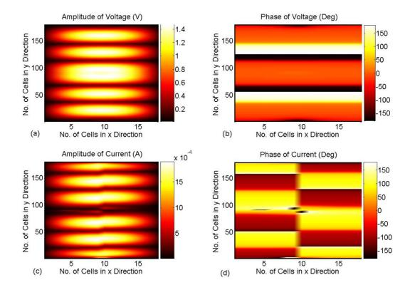
The voltage and current distributions on the planar TL-metamaterial super waveguide with  $18 \times 179$  unit cells computed by TMM. (a) The amplitude distribution of voltage. (b) The phase distribution of voltage. (c) The amplitude distribution of current. (d) The phase distribution of current.
