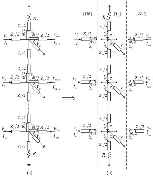
The equivalent-circuit T network for a column cell and the corresponding decomposition. (a) T network for a column of cell. (b) The decomposition of three parts.
