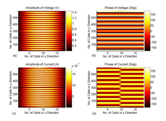
The voltage and current distributions of a longer TL-metamaterial super waveguide with 18 × 599 unit cells computed by TMM. For the same structure, ADS cannot be used due to the memory limit of personal computer. (a) The amplitude distribution of voltage. (b) The phase distribution of voltage. (c) The amplitude distribution of current. (d) The phase distribution of current.
