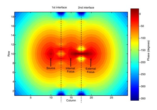
**Figure 5** TMM-simulation results for TL super lens [9] at 1 GHz (voltage phase).
