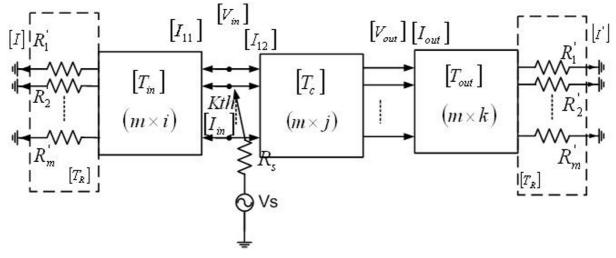
The whole network under consideration, including *m* inputs and *m* outputs, which is divided into the input network  $T_{in}$ , the center network  $T_c$ , and the output network  $T_{out}$ . A source is arbitrarily located at the *k*th row and between the *i*th and (*i* + 1)th columns of the network.
